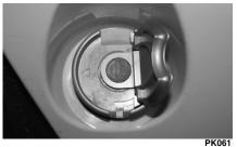
After filling the tank, position the lid towards the right side of the filler neck and rotate the lid ¼ turn clockwise to secure. Flip the lid up.
