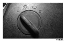
With the ignition switch in the ON position, use the headlight switch to select off, running, low, or high beam.
