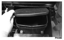
4. To open the tailgate compartment, pull outward on the locking lever and allow the tailgate storage cover to pivot downward. To secure the tailgate storage cover, pivot the cover upwards and press firmly on both left and right hands sides.
