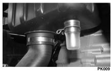
14. Insert the air filter screen into the inner element; then secure the air filter holders with the Phillips screw.
