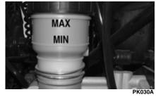
Check the brake fluid level in the brake fluid reservoir. The fluid level must be maintained between the MAX and MIN level marks. If the
