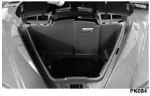
2. To open the glove box (if unlocked), squeeze the locking tabs together and pivot the lid downward or insert the key and rotate 1/8 turn counterclockwise and pivot the lid downward. To lock the glove box, close the lid, insert the key, and rotate it 1/4 turn clockwise. Remove the key.
